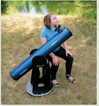
calculate magnification by dividing the eyepiece focal length into the telescope's focal length. For instance, a 900-mm telescope with a 25-mm eyepiece gives you  $36\times - (900/25 = 36)$ .
