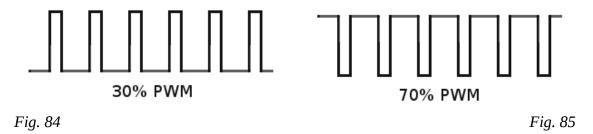
strip powered on 30% will radiate less heat into the optics.
