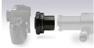
Figure 79 shows the Williams Optic Flattener III reducer flattener. This unit has a camera's T adaptor incorporated into it and reduces the focal length to 80% of original; so an f/6 refractor would become an f/4.8 refractor with the field flattened. It will work for many telescopes.
