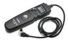
Once everything is setup, aligned and it's dark out it's time to start taking images. This means that some method of exposure control has to be in place. Whether this is simply a manual remote and a wrist-watch (not too accurate) or something a bit more complex the shutter has to open and close when needed. Those using CCD cameras will have the camera control software running on a computer so I won't dwell on these and move on to DSLRs.
